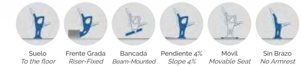
Suelo To the floor Frente Grada Riser-Fixed Bancada Beam-Mounted Pendiente 4% Slope 4% Móvil Movable Seat Sin Brazo No Armrest
